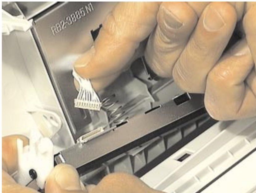
Figure 4-6 Disconnecting the CIS wire connector
