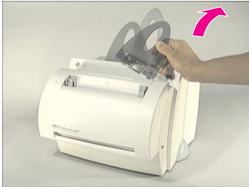
Figure 4-1 Removing the paper guides
