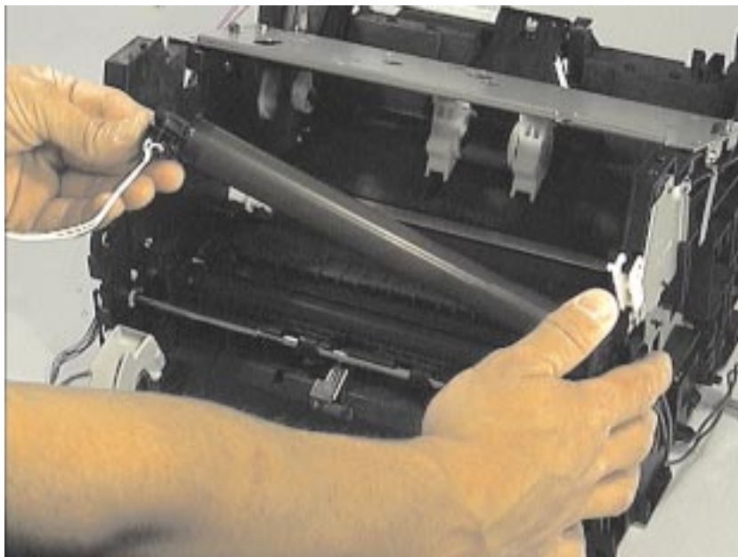
Figure 4-31 Removing the fusing element
